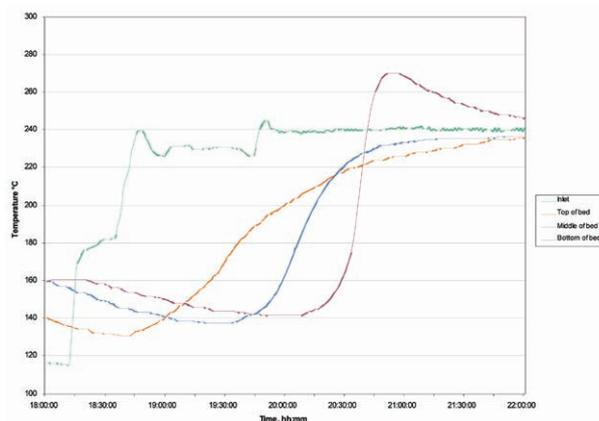
Figure 5. SCOT-reactor temperature profiles during in-situ presulfiding process.
