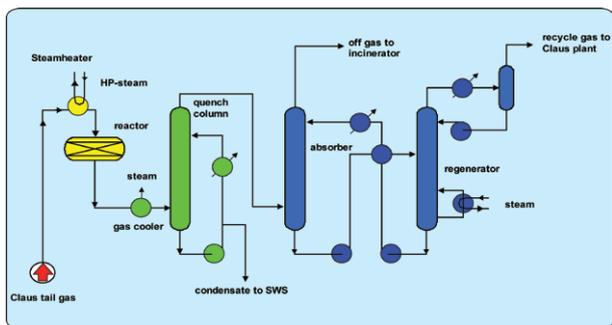
Figure 1. Low temperature tail gas treating with steam reheater.
